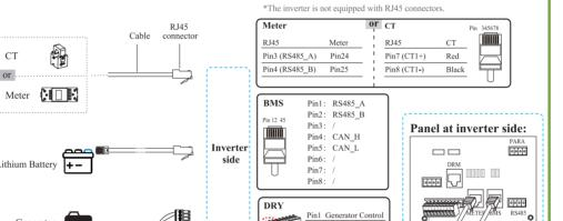
① Assemble the communication cables with an RJ45 connector/9-Pin terminal according to applicable Pin definition ②Insert these cables into corresponding communication ports according to panel at inverter side.
